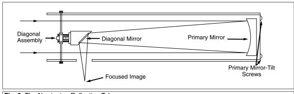
Fig. 6: The Newtonian Reflecting Telescope.
